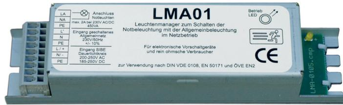
The lamp manager unit LMA01 is intended for use with: **BK, BX, ZX, ZDCL** and **MULTI-CONTROL**. With this unit it is possible to operate maintained lamps and backup lamps at the same time, if SKML are used. A lamp load with a maximal load of 2A connected to the emergency light exit is supplied in case modified readiness with mains AC, otherwise it/they is/are in non-maintained mode.
